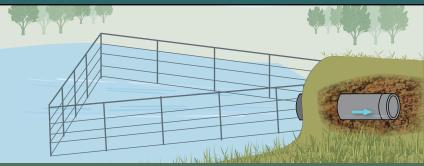
**Exclusion devices** (shown above) – constructed fencing to keep beaver activity away from culverts and tile outlets
