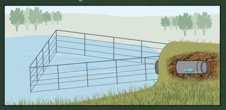
**Exclusion devices** (shown above) – constructed fencing to keep beaver activity away from culverts and storm drains
