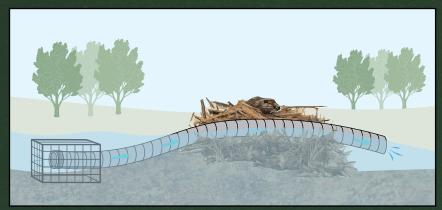
**Deceiver on upstream main dam** (shown above) allows water to flow through dam
